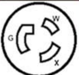
NEMA L5-20 120 volt, Single Phase 3 wire, grounding 20 amp
